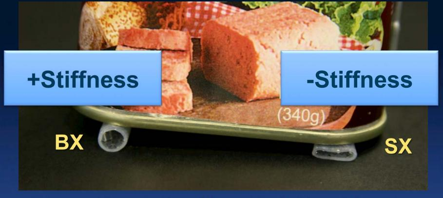
BX stent withstands 12oz of Corned Beef without deformation SX stent flattens under Corned Beef load...
