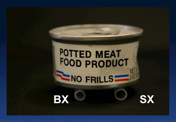
BX stent and SX stent withstand 3oz of P.M.F.P. without deformation
