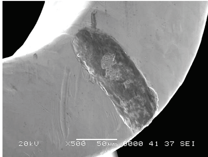
Figure 7: Wear damage on stainless steel stents after 10 million cycles axial fatigue testing (worst case).
