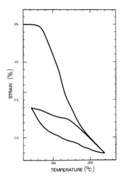
FIG. 5 Strain shown as a function of temperature after an initial tensile deformation of e = 3.4 %. Initial heating produces a 50 % recovery of the original 3.5 % strain, subsequent cooling and heating produces a closed "two-way" hysteresis loop.
