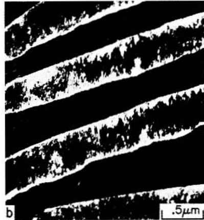
Figure 13. Sympathetically nucleated \alpha in Ti-10-2-3 \beta -solution treated and aged at 600°C. a) light micrograph, b) TEM micrograph.
