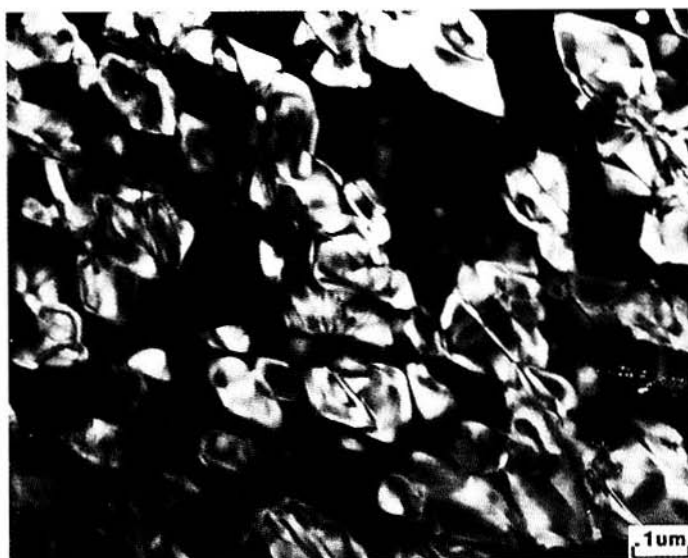
Figure 10. Ledges forming upon cuboidal \omega in a Ti-V alloy during final stages of \omega -phase stability.
