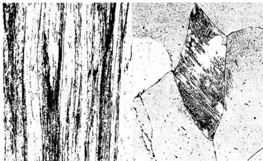
Fig. 5: Preheating temperature 825°C, deformation velocity 4 mm/s, as-forged condition. The right picture shows the surface and the left the center. 225x. Geometry and material as in Fig. 4.
