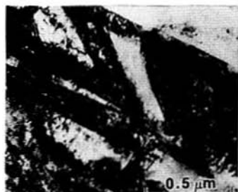
Figure 9: Bright field image show self-accommodation of strain martensites.
