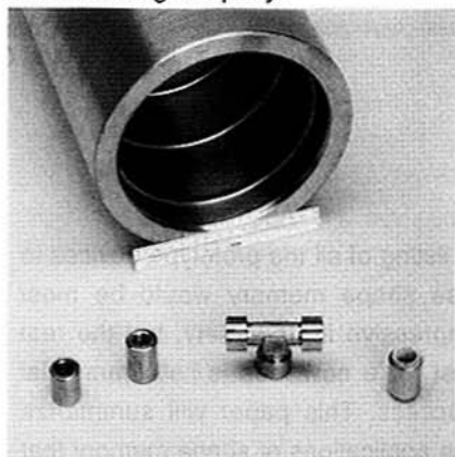
Figure 3: The four basic types of marine coupling are shown in front of the largest coupling ever made: a Ni-Ti-Fe coupling used for joining 15 mm diameter subsea gas lines.
