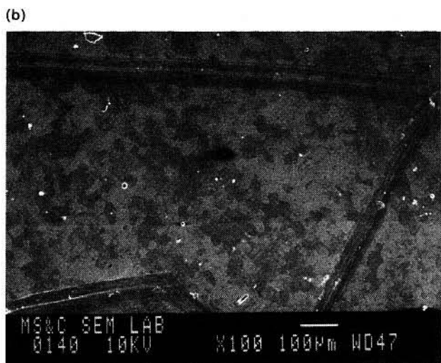
Figure 9. (a) SEM micrograph of a sputter-cleaned surface. The scratch was artificially introduced on the surface to mark a particular area for analysis. (b) SEM micrograph of the surface shown in (a) after 1 min in air at 450 °C.
