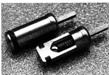
Fig. 5. Thermostatic oilcooler by-pass valve for automatic transmission
