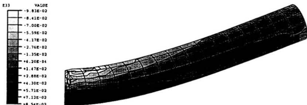
Figure 5: FEA model of 1.5mm diameter wire at 2.7mm deflection under 3-point bending.
