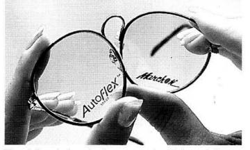
Figure 5: Superelastic eyeglass frames are constructed of superelastic temples, nose bridge, and often a brow piece. Components are brazed and welded to Monel or German Silver, then often polished and gold plated.
