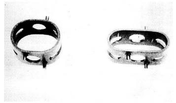
Figure 7: Spinal vertebrate spacer shown in the martensitic state (left) and deployed superelastic state (right). The properties of Nitinol promote more rapid recovery due to the similarity of mechanical properties between the implant and the surrounding tissue.
