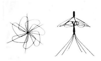
Figure 3: Simon Filter, shown in longitudinal and transverse views of the deployed state, is the first class III Nitinol implant approved by the FDA (the function of the device is described later).
