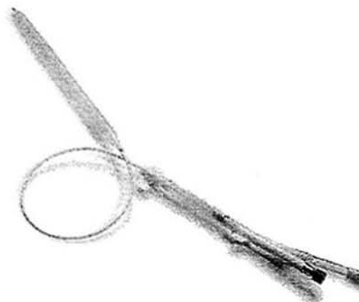
Figure 7: Arrow Intra Aortic Balloon catheter which uses kink resistant Nitinol tubing to allow movement through tortuous paths into the heart chamber. The device is used to provide back pressure to assist heart beating.
