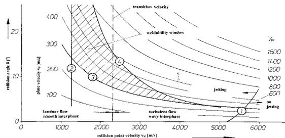
Fig. 2 Explosive weldability window, schematic
