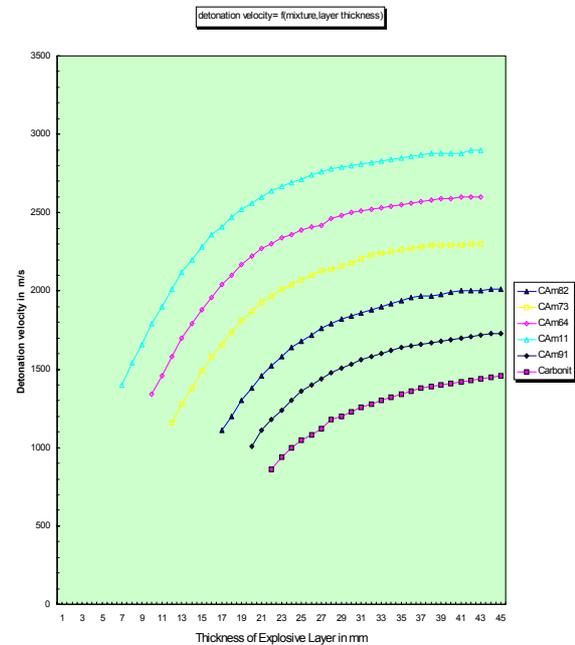
Figure 3 Detonation velocity of different kind of explosives as a function of layer thickness. CA91 = ratio of Carbonit and Ammonit = 9 : 1.
