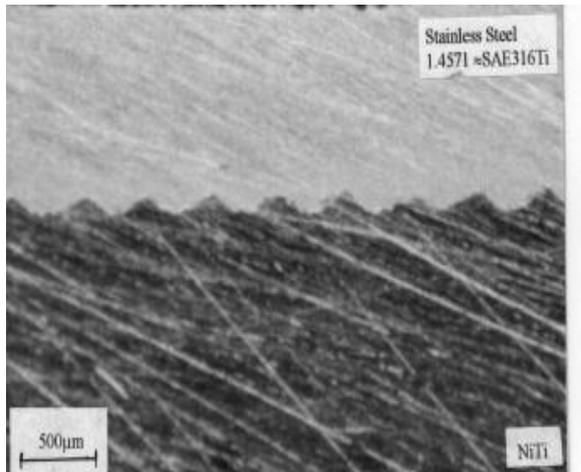
Figure 4. Wavy interphase of explosively welded NITINOL- Stainless Steel compound, welded at a collision point velocity of 2580 m/s
