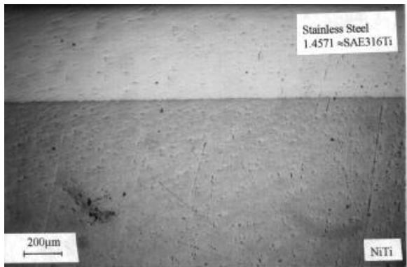
Figure 5. Smooth interphase of explosively welded NITINOL- Stainless Steel compound, welded at a collision point velocity of 2190 m/s
