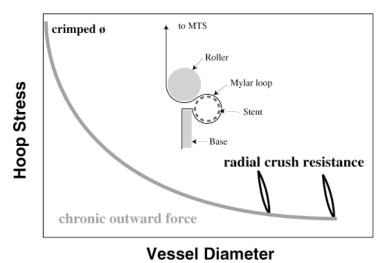
Figure 3. Schematic radial force test set up
