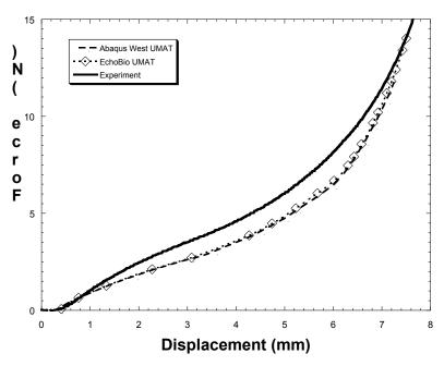
Figure 10. Comparison of force-displacement relations from experiment and FEA
