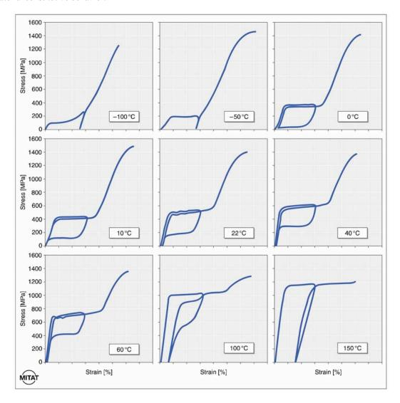
Figure 1. Uniaxial stress-strain relation at different temperatures
