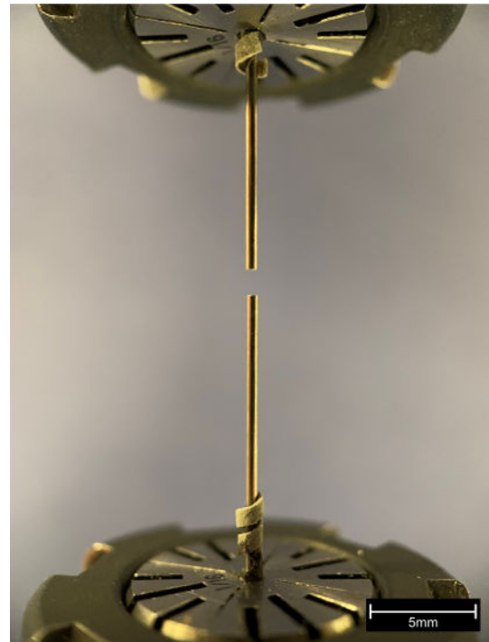
Fig. 7. Image of a FIB-milled wire test specimen that had fractured from the gauge section under axial tension-tension fatigue. The fracture had originated at the FIB-milled starter crack. The specimen depicted in the image fractured at 4.22 million cycles.
