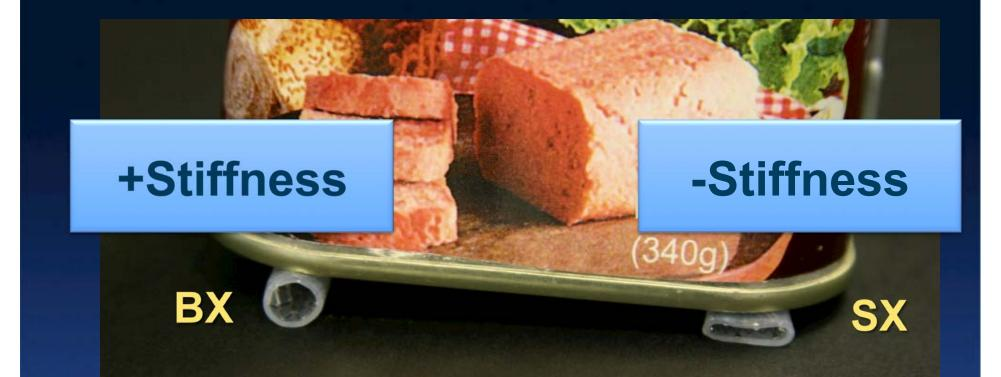
BX stent withstands 12oz of Corned Beef without deformation SX stent flattens under Corned Beef load...
