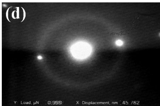
Fig.4 Engineering stress vs. displacement curve (a) and corresponding diffraction patterns (b-d) from a compression test with 15% nominal engineering strain. The video frames (b-d) correspond to the points marked on (a), and in each case the frame corresponding to the end of an event is shown in order to show the full intensity of the
