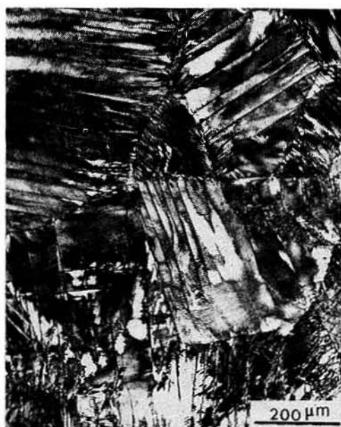
Fig. 14. Optical micrograph showing microstructure after deformation (2.5%) and slowly heating to 620°C.
