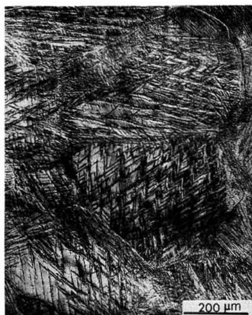
Fig. 4. Microstructure after 2% plastic deformation.
