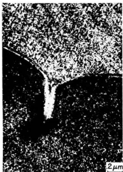
Figure 15. TEM micrograph showing an example of how inclusions can pin \beta grain boundaries.
