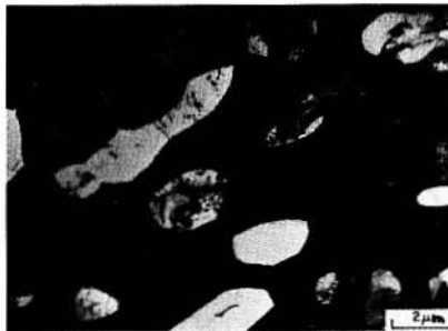
Figure 2. Bright field TEM micrograph showing typical bimodal microstructure of a lean \beta titanium alloy. The coarse, globular primary \alpha is light colored and monolithic, the fine acicular \alpha in the surrounding \beta -matrix is visible only via TEM. This particular microstructure is that of Ti-10-2-3 after \alpha + \beta solution treating at 720^\circ\text{C} for 2 hrs and then aging at 400^\circ\text{C} for 1000 m.
