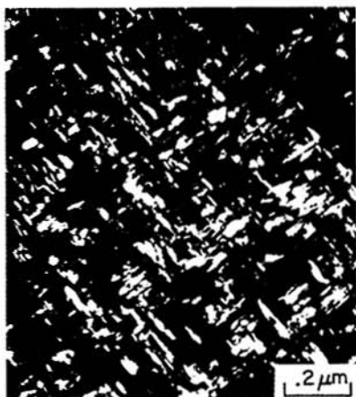
Figure 11. Typical fine, stubby \alpha -phase that results from nucleation in an \omega -phase dispersion. (Ti-10-2-3 \beta -solution treated and aged 1 h at 500°C).
