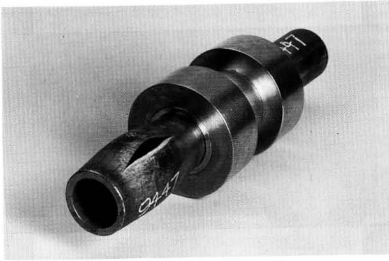
c) Installed and burst on 2.375" pipe.
