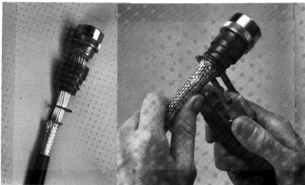
Figure 3: A backshell connector using a shape memory alloy ring.
