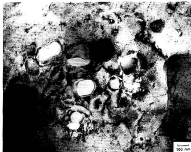
Fig. 5—Microstructure of RSP Al-10 pct Be-3 pct Li ribbon heat-treated at 185 °C for 1 h.
