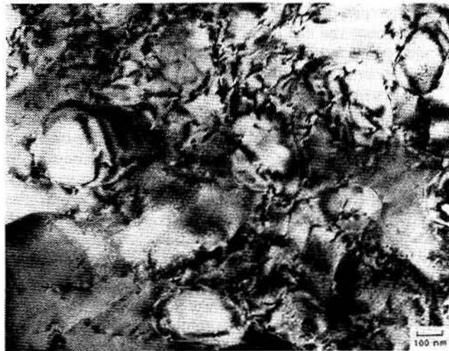
Fig. 2—Microstructure of an RSP Al-10 pct Be-3 pct Li ribbon heat treated at 405 ^{\circ}\text{C} for 0.5 h. There are three precipitate phases present in the matrix: \alpha -Be, \delta' , and \delta .
