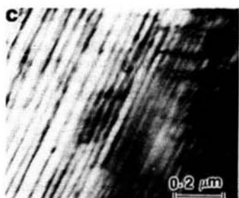
Figure 7: Internal defects of martensites in \text{Ni}_{47}\text{Ti}_{44}\text{Nb}_9 alloy at -105^\circ\text{C} . (a) Bright field image of twin martensite (b) Corresponding electron diffraction pattern (c) Bright field image of martensite showing stacking faults (d) Corresponding diffraction pattern
