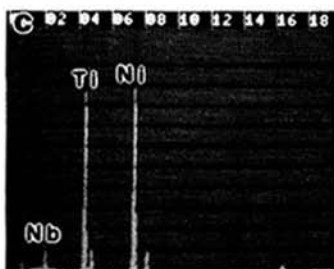
Figure 2: (a) Transmission electron micrograph of \text{Ni}_{47}\text{Ti}_{44}\text{Nb}_9 alloy annealed at 850^\circ\text{C} for 30 min, (b) (c) corresponding EDX spectra taken from precipitate labeled P in (a) and matrix labeled M in (a), respectively
