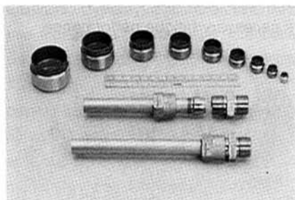
Figure 2: Cryolives® use a Ni-Ti-Fe sleeve shrunk unto tubing to provide a demateable high performance joint.
