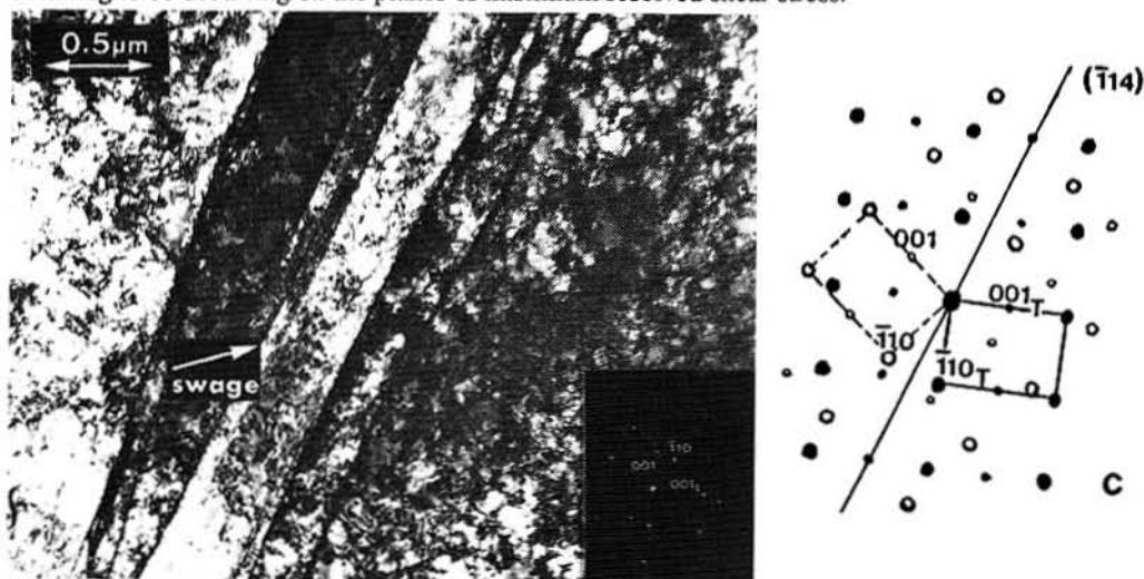
Figure 1. \{114\} complex mechanical twinning in 10% cold swaged B2 intermetallic. Figure 1b and 1c. Electron diffraction, and schematic, of \{114\} twin plane at \sim 43^\circ to the swaging axis.
