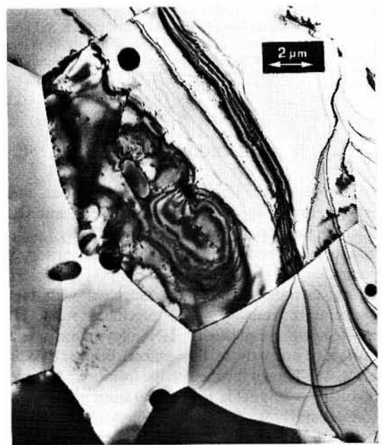
Fig. 1. Bright field image of microstructure of \text{Ti}_{50}\text{Ni}_{47}\text{Fe}_3 alloy after annealing 2 h at 875°C. The nominal grain size is \sim 40 \mu\text{m} .
