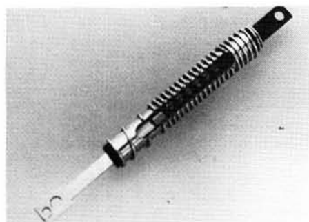
Figure 12. The VEASE® actuator was designed to be a complete electrical actuator package; an overload spring on the outside of the device protected the memory spring from deforming itself. (Raychem)
