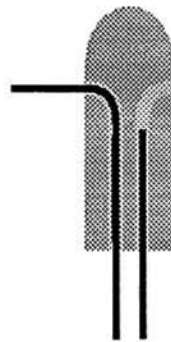
Fig. 10: Catheter tip with side-deploying needles [12]
