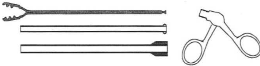
Figure 6: Modular design of hingeless instruments
