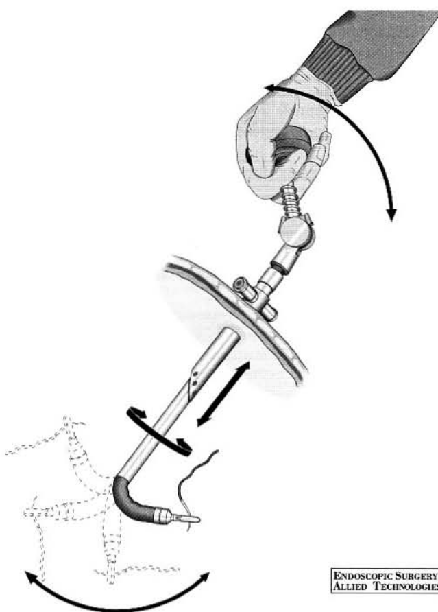
Figure 9 a, b: Endoscopic suturing by means of experimental dextrous instruments and needle drivers (developed in co-operation with the Nuclear Research Centre, Karlsruhe, Germany) permits the whole range of required needle positions relative to the tissue defect. However, adequate needle friction is difficult to achieve and the process requires considerable training.
