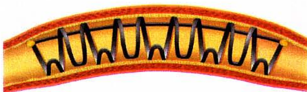
Figure 6. Cook GR1. Formed from stainless steel sheet, featuring an axial backbone with integral gold markers
