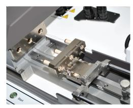
Confluent Medical recommends purchasing the CPS-1000 parison stretcher in tandem with the Confluent Medical BFM-4410. The CPS-1000 has enhanced software built-in that adds a parison conditioning step to insure blowing the balloon from the center for ideal results.
